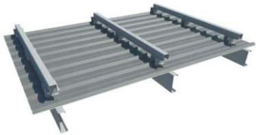
"Ω"Shape Purlin Installation
