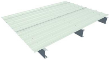
Bottom Panel Installation
